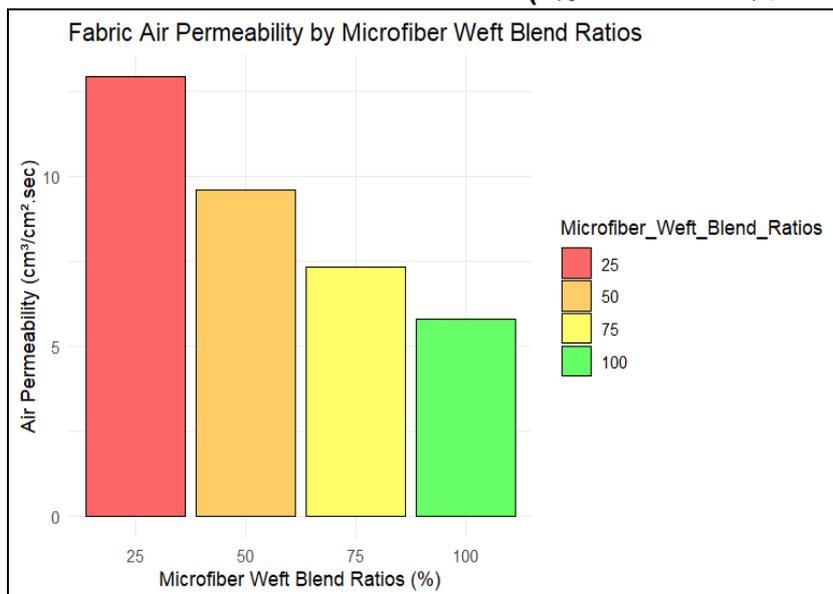
**FIGURE (11) RELATIONSHIP BETWEEN MICROFIBER WEFT BLEND RATIOS AND FABRIC AIR PERMEABILITY**
