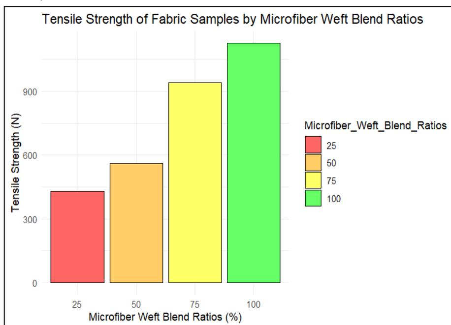
**FIGURE (6) RELATIONSHIP BETWEEN MICROFIBER WEFT BLEND RATIOS AND FABRIC TENSILE STRENGTH IN THE WEFT DIRECTION**
