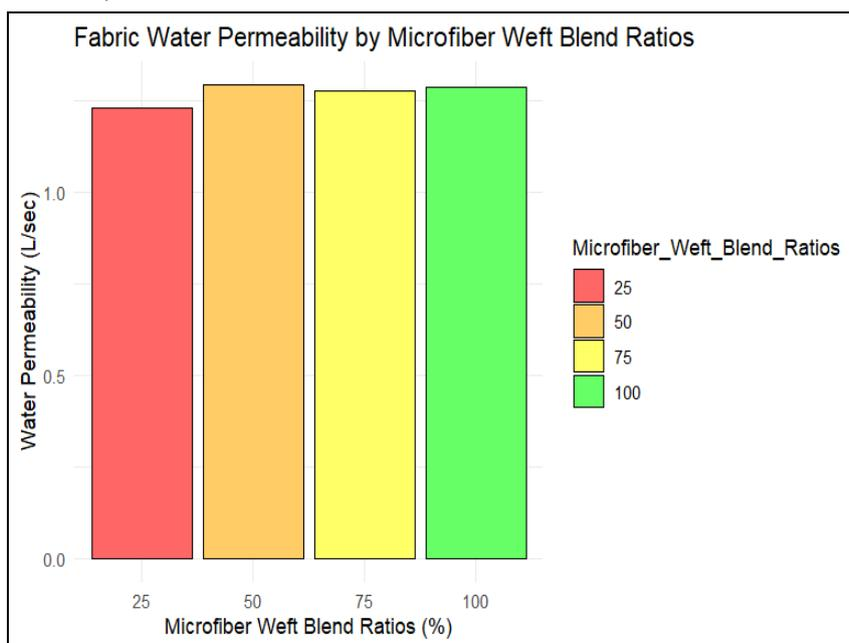
**FIGURE (12) RELATIONSHIP BETWEEN MICROFIBER WEFT BLEND RATIOS AND FABRIC WATER PERMEABILITY**
