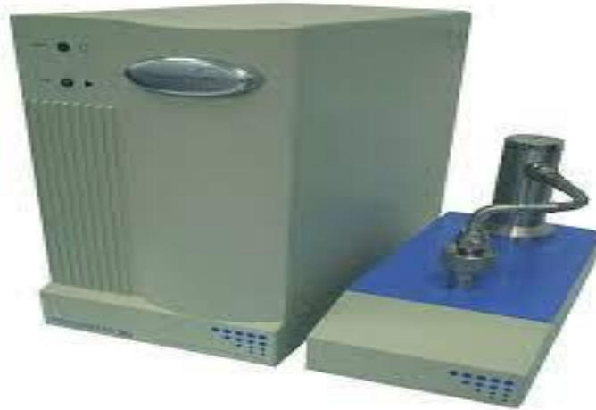
Figure 3: Photo of the porosity meter used
