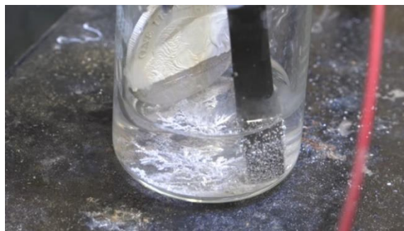
Figure5. the cathode just starts to bubble hydrogen
