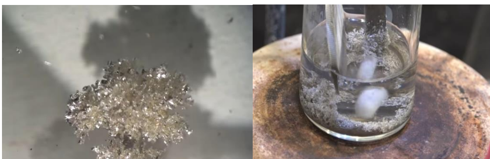
Figure6. The silver dendrites are growing.
