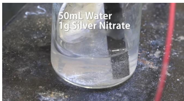
Figure2. Solution of 1g silver nitrate in 50 ml water
