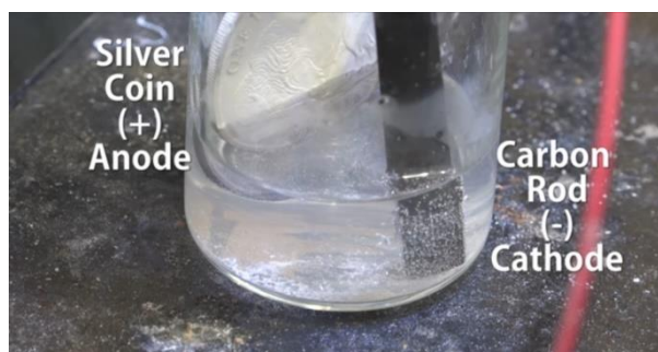
Figure4. Connect the anode (silver) and the cathode (carbon)
