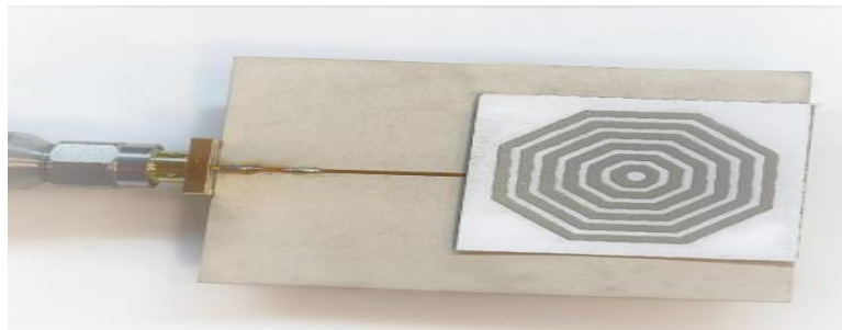
Figure 26. Near field RFID tag identification printed on paper by using a wideband antenna
