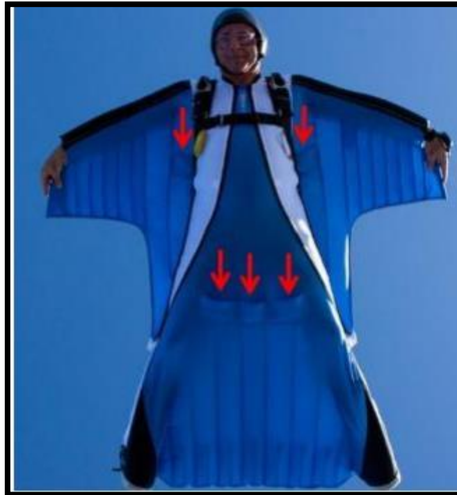
FIGURE 7: WINGSUIT INLETS ARE POSITIONED TO RECEIVE RAM-AIR TO PRESSURIZE THE AIRFOIL SHAPES OF THE SUIT. THEY CAN BE SEEN UNDER THE ARMPITS AND BETWEEN THE LEGS OF THE WINGSUIT SHOWN BY RED ARROWS ABOVE (TONYSUITS 2010)
