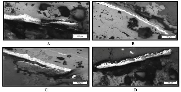
Fig. (3) A, B, C and D metallographic photomicrographs of the copper tray samples show corrosion layers and erosion of copper with clay and quartz minerals.
