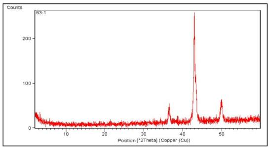
Fig. (6) Shows XRD pattern of corrosion sample.
